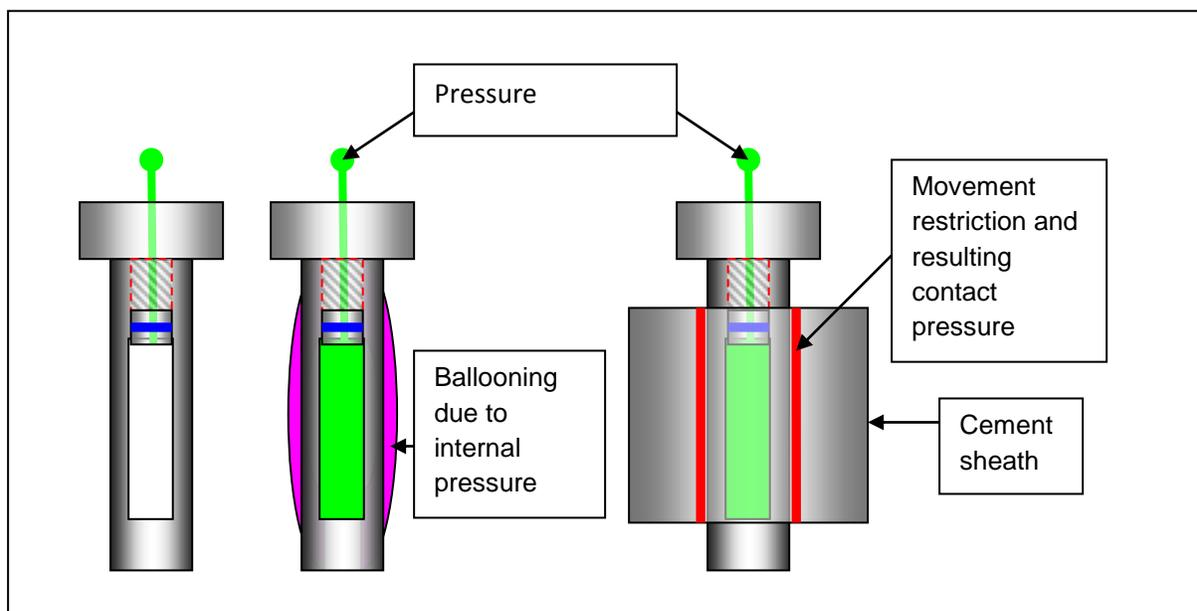
Figure 9: Ballooning Effect as Reason for the Stresses in the Cement
