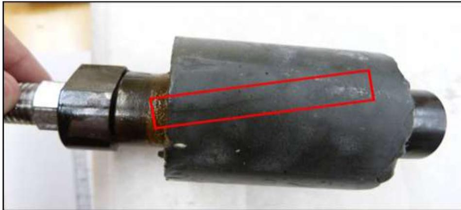
Figure 10: Cement Failure with Low Curing Time
