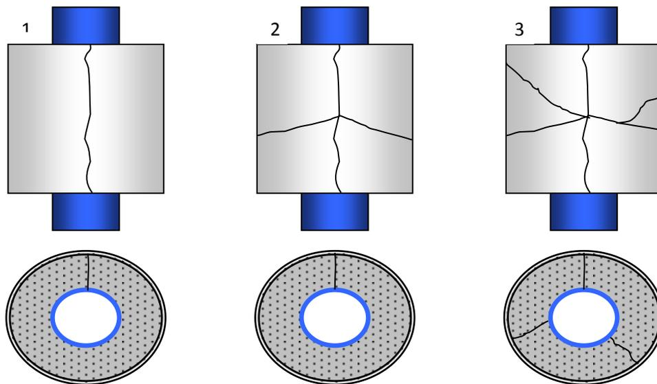
Figure 12: Phases of Cement Failure [4, 13]
