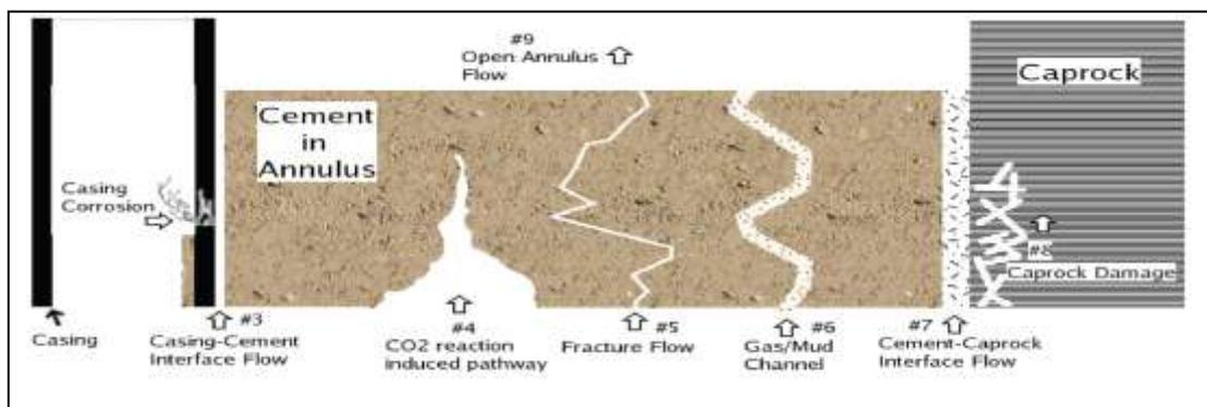
Figure 2: Cement Failure Modes Summary [5]
