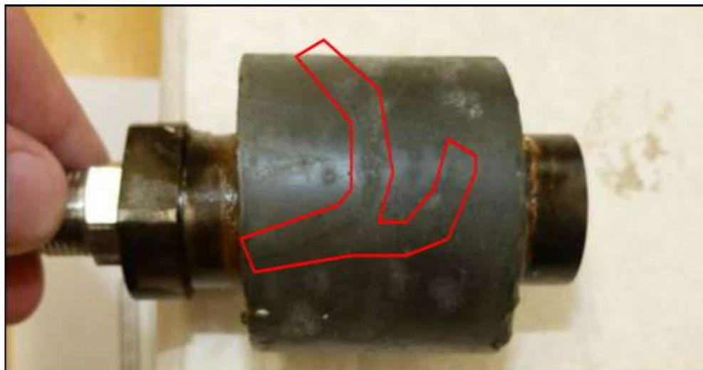
Figure 11: Cement Failure as Network from Initial Crack
