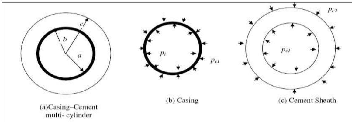
Figure 4: Geometry and Assumptions in the Analytical Model by Ugwu and Teodoriu [11, 12]
