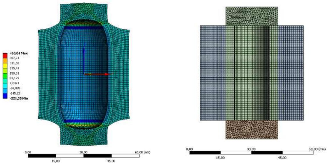
Figure 8. The deformed shape of the specimen (left) versus its original shape (right)
