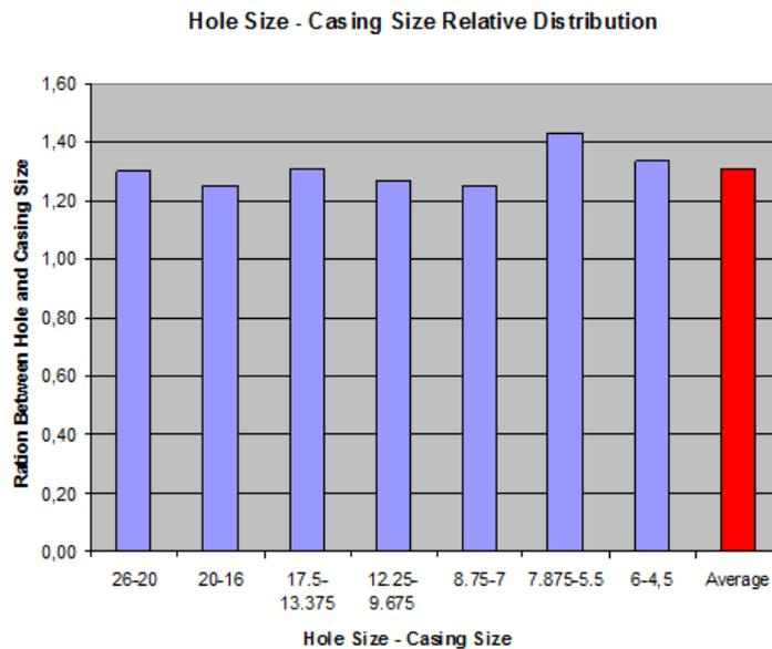
Figure 5. Ratio between hole and casing size, used to estimate the cement sheath behavior, using API recommended casing – hole size pairs [1]
