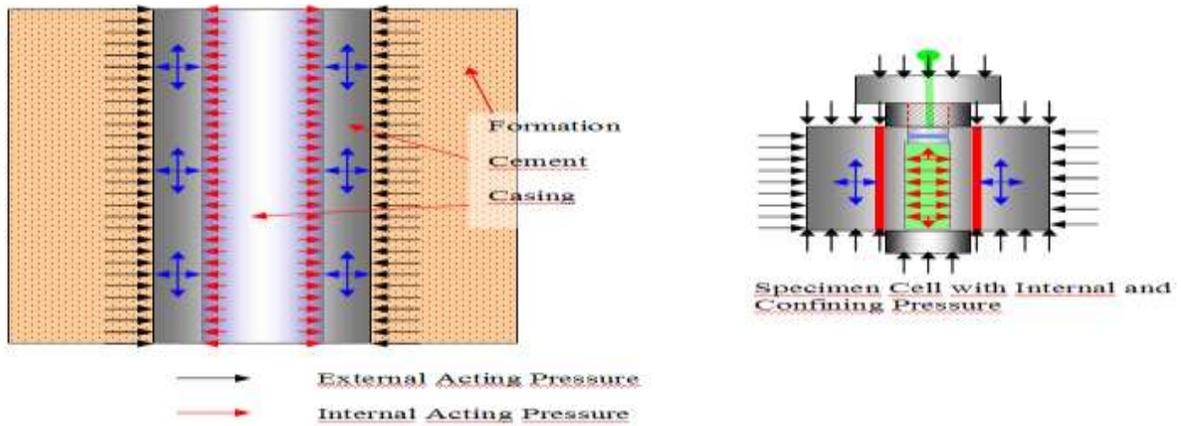
Figure 7. Real versus Laboratory loads on a cement sample
