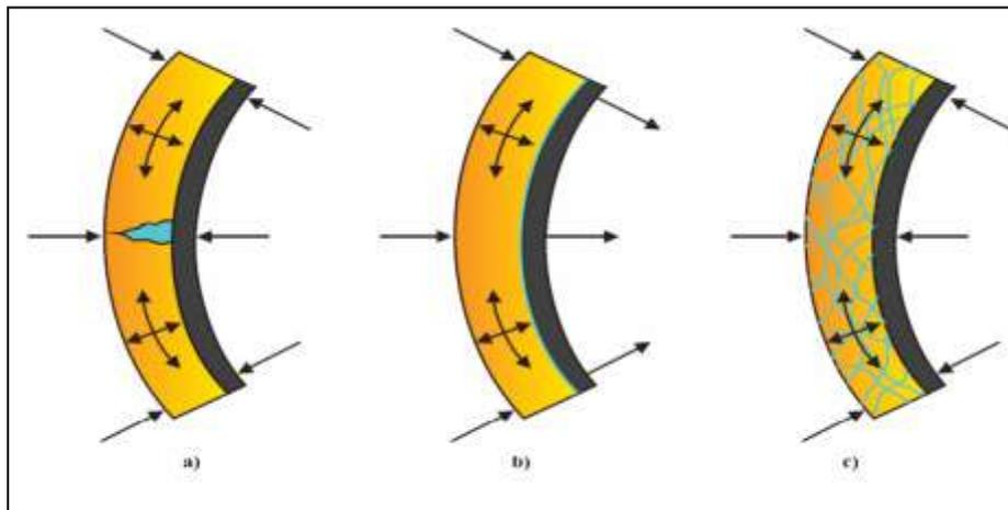
Figure 3: Types of Mechanical Cement Failure a) Radial Crack b) De-bonding c) Shear Failure, (Wehling 2008)
