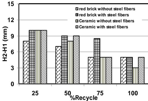
Figure (21) Flow Time and % Recycling Relationship for J-Ring Test.
