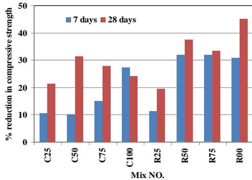
Figure (6) Reduction in compressive strength of recycled self-compacting concrete.
