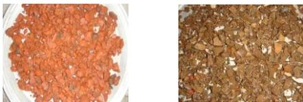
(a) Crushed red brick agg. (b) Crushed ceramic agg.
