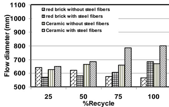
Figure 20) Flow Diameter and % Recycling Relationship for J-Ring Test.
