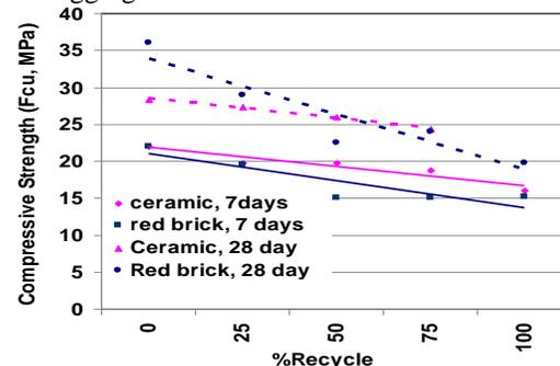
Figure (5) compressive strength for recycled self-compacting concrete.
