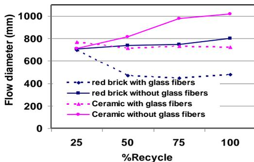
Figure 18) Flow Diameter and % Recycling Relationship for Slump Test.
