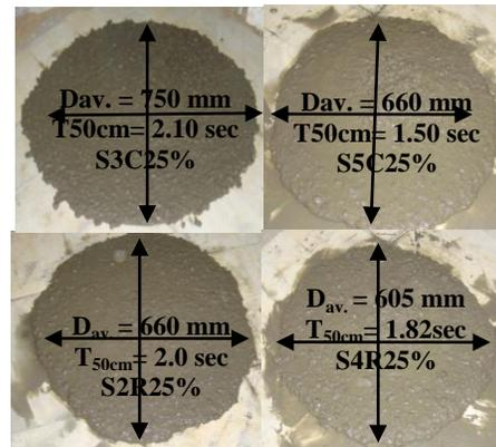
Figure (9) Flow Diameter for GRSCC Mixes.
