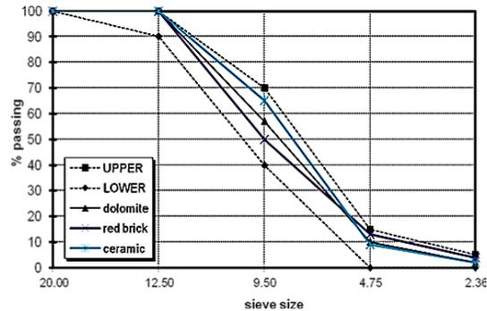
(c) Grading of coarse aggregate
