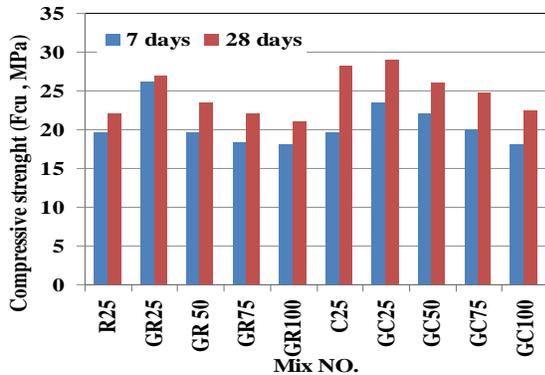
Figure (22) Compressive Strength of GRSCC
