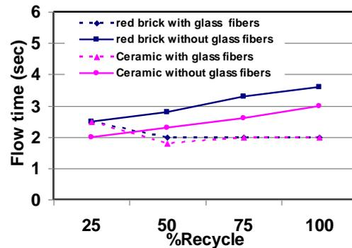
Figure 19) Flow Time and % Recycling Relationship for Slump Test.
