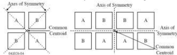
Figure 14. Common centroid layout
