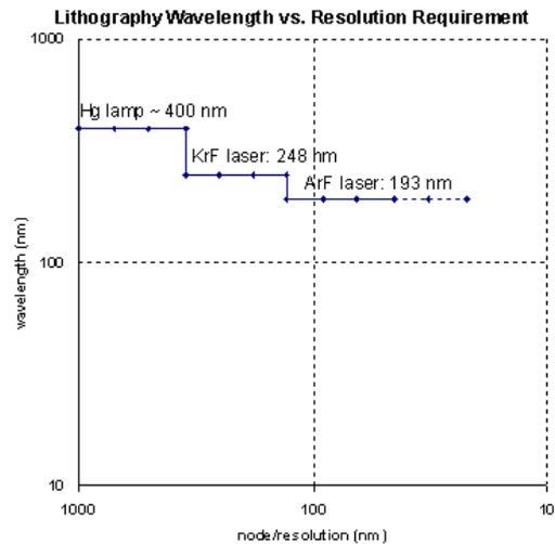
Figure 5. Photolithography photon's wavelength vs resolution.
