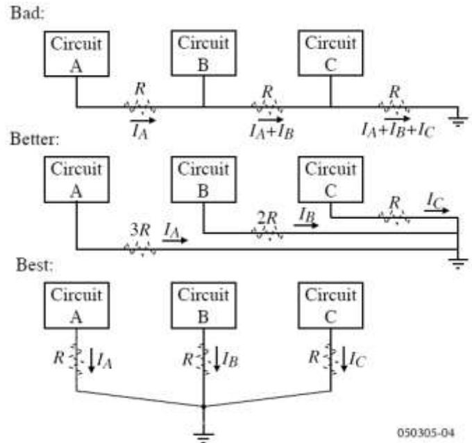
Figure 15. Layout for minimization of the parasitics' effects in ground connections
