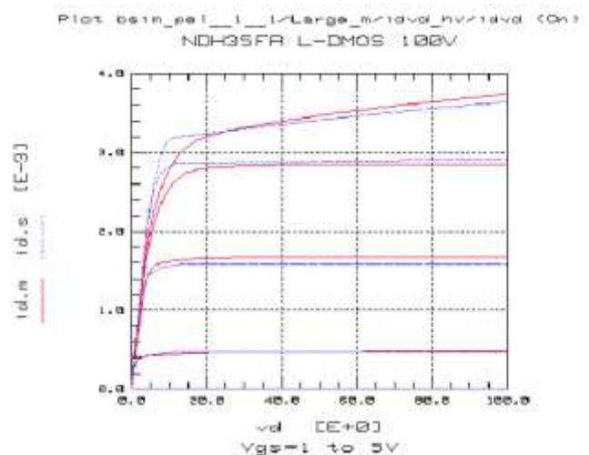
Figure 13. Simulated (blue) vs measured (red) Ids-Vds characteristics of an N-type HV transistor
