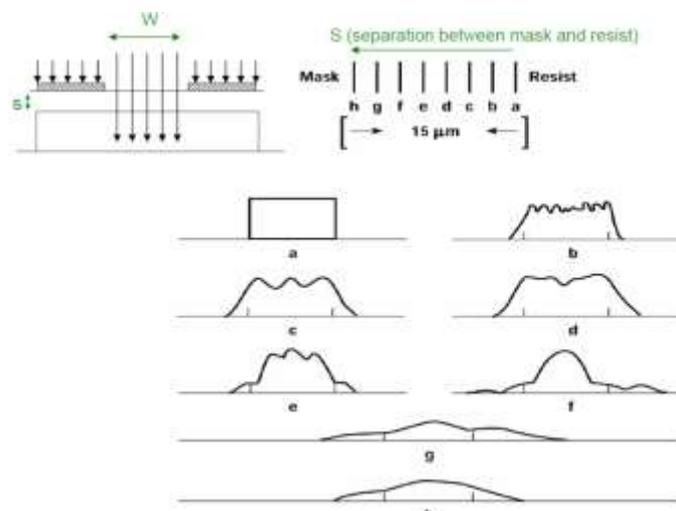
Figure 7. The effect of light diffraction on photoresist pattern formation.
