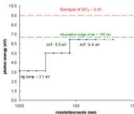
Figure 4. Photolithography photons' energy vs resolution.
