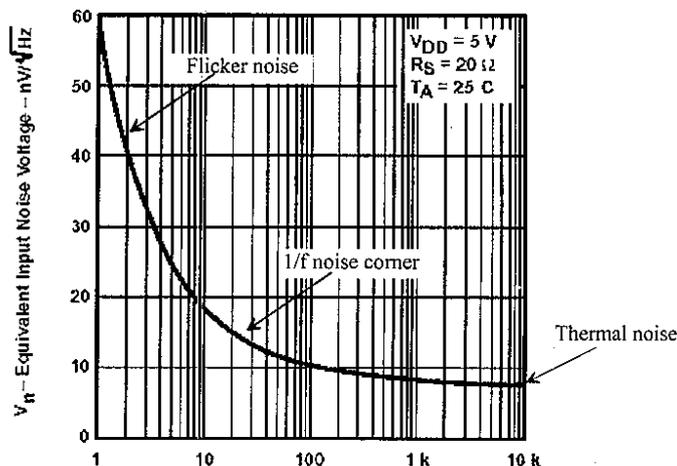
Figure 2. Noise frequency spectrum of a real semiconductor device.
