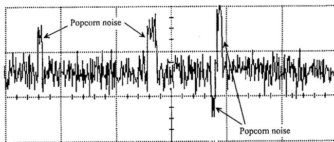
Figure 3. Burst noise waveform.
