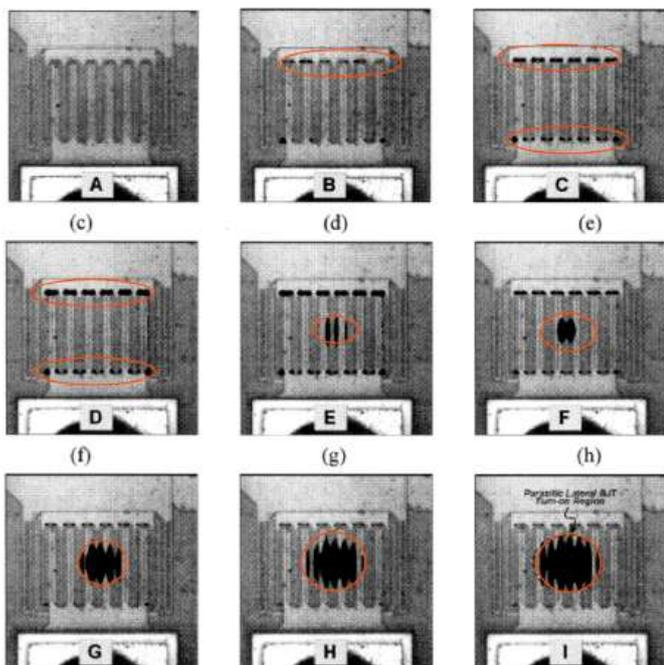
Figure 1. Photon generation of the NMOS under direct voltage.
