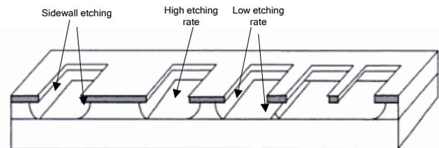
Figure 8. Etching hazards.
