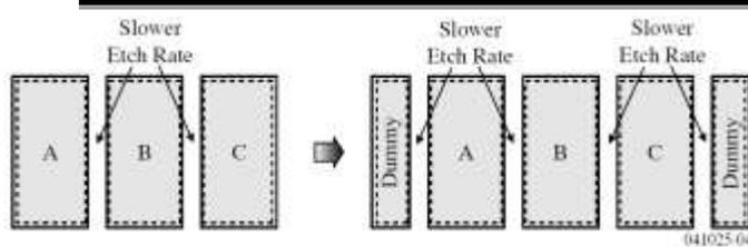
Figure 17. Layout for a uniform etching.
