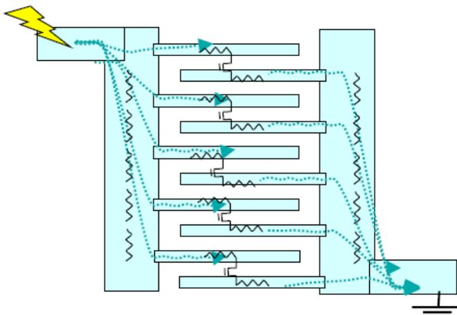
Figure 9. MOSFET layout with hot spot reduction
