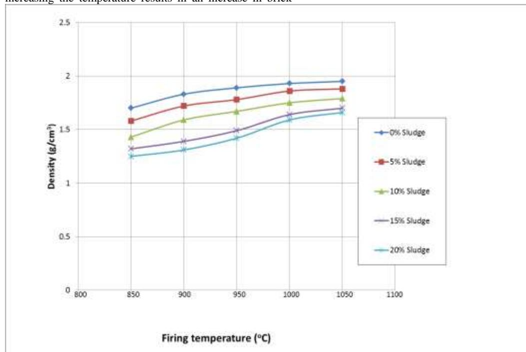
Fig. 4. The density of sludge-clay burnt bricks
