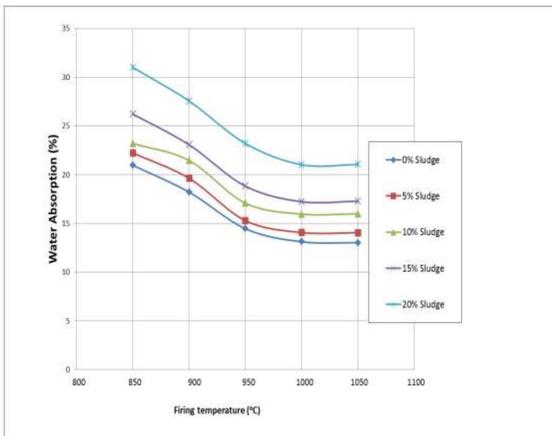
Fig. 3. The water absorption of sludge-clay burnt bricks
