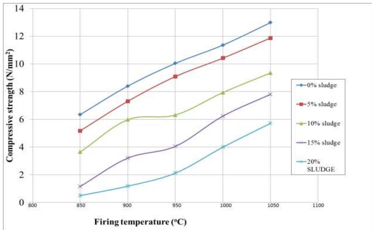
Fig. 2. The compressive strength of sludge-clay burnt bricks.
