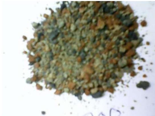
Plate II: Processed Sludge at 700°C
