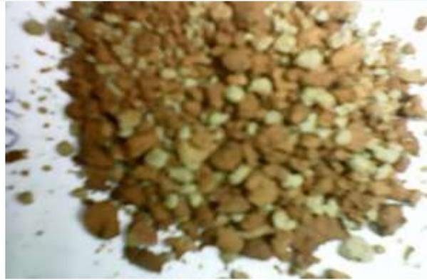
Plate IV: Processed Sludge at 900°C
