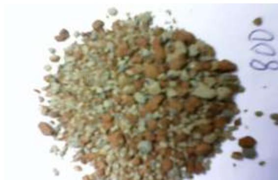
Plate III: Processed Sludge at 800°C
