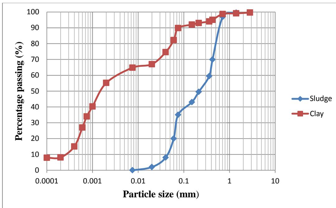
Fig. 1: Particle Size Distribution of LUDWTP sludge and clay
