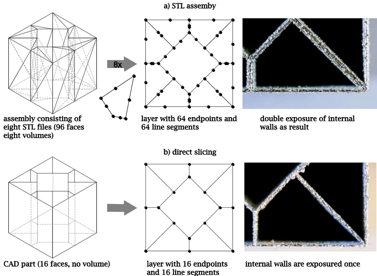
Figure 7: Thin walled design approaches
