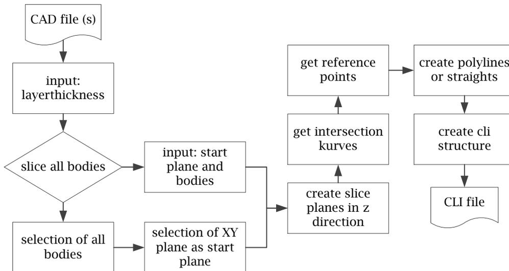
Figure 8: KF based direct slicing in NX
