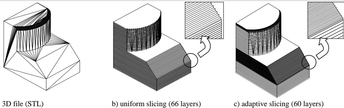
Figure 4: Comparison of uniform (b) and adaptive slicing (c) based on STL geometry (a)
