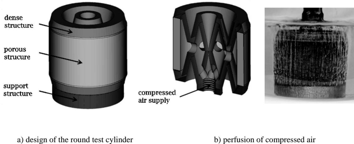
Figure 1: Round test cylinder [4]
