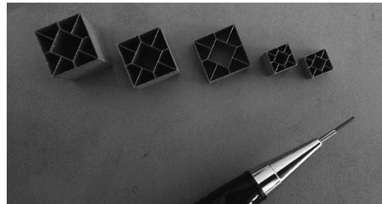
Figure 2: Test geometry for thin walled elements
