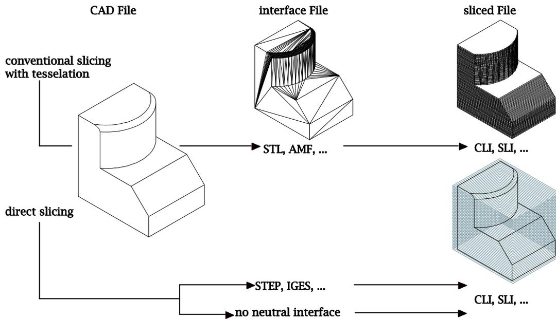
Figure 3: Conventional and direct slicing
